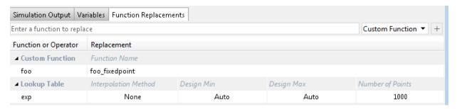
You can add and remove function replacements from this list. If you enter a function replacement for a function, the replacement function is used when you build the project. If you do not enter a replacement, the app uses the type specified in the original MATLAB code for the function.
